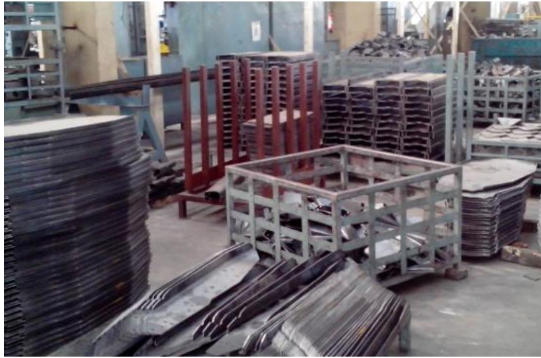
Fig4.6: Figure of improper arrangement of raw material after first cutting
